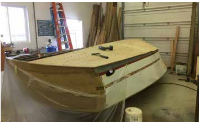
Above: Work in progress for a new bottom panel for the "Al dZine," a 1959 Gyded Missel.
