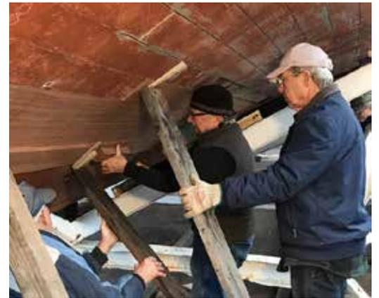
*Top: Bob assisted on repairs for PT 658 and cleaning up after removal of the STBD muffer to facilitate replacement of deteriorated planking during the 2018-2019 PT 658 haul-out. Bottom: Working with other volunteers and shipwright, Jim Lyons, Bob helped with the fitting of new planks during the 2018-2019 PT 658 haul-out.*
