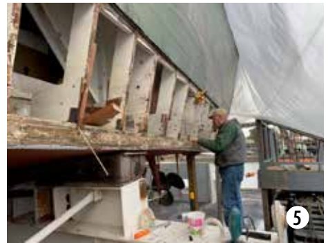
Photo 1: The PT 658 in its cradle aboard the barge on Swan Island undergoing maintenance and repairs. Photo 2: Side frames were repaired by fitting a new stub frame and adding a "sister" to overlap the joint. Photo 3: Shipwright Jim Lyons installs fasteners into a new plank. Photo 4: Volunteer Steve Stange installs plugs over the new screws. Photo 5: Volunteer John Kihlstrum prepares damaged frames for repair.
