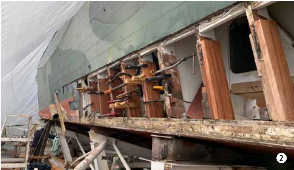
Photo 1: The PT 658 in its cradle aboard the barge on Swan Island undergoing maintenance and repairs. Photo 2: Side frames were repaired by fitting a new stub frame and adding a "sister" to overlap the joint. Photo 3: Shipwright Jim Lyons installs fasteners into a new plank. Photo 4: Volunteer Steve Stange installs plugs over the new screws. Photo 5: Volunteer John Kihlstrum prepares damaged frames for repair.
