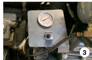
Photo 1: PT 658 was seen with a group of guests on board to meet the ships arriving for Portland's Fleet Week. Photo 2: New engine pre-oiler pumps were installed below-deck to each of the three Packard V12s engines. Photo 3: The recently installed PT 658 lubrication system pre-oiler control panel is below-deck.
