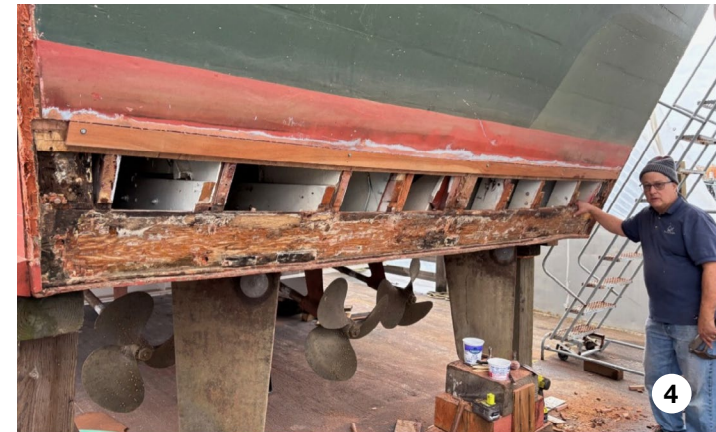
Photo 1: PT 658 is in drydock and tarped to keep crew and boat dry. Photo 2: CWC member, Ian Harding, and shipwright, Jim Lyons, were laying out a new plank using the pattern made from the boat. Photo 3: Jim Lyons rough-cut a new plank with help from volunteer John Kihlstrum. Photo 4: CWC member and PT 658 volunteer, Don Cameron, made repairs to the transom framing prior to installing new inner and outer planking.
