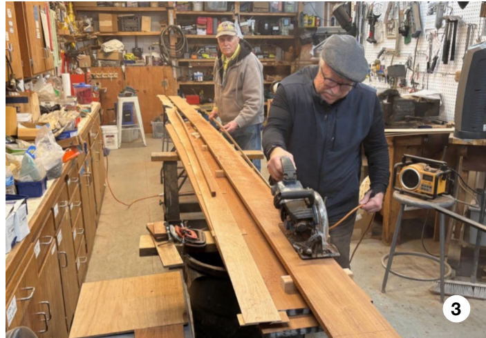
Photo 1: PT 658 is in drydock and tarped to keep crew and boat dry. Photo 2: CWC member, Ian Harding, and shipwright, Jim Lyons, were laying out a new plank using the pattern made from the boat. Photo 3: Jim Lyons rough-cut a new plank with help from volunteer John Kihlstrum. Photo 4: CWC member and PT 658 volunteer, Don Cameron, made repairs to the transom framing prior to installing new inner and outer planking.
