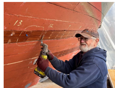
Above: PT 658 Volunteer Gary Veenker trimmed wood plugs installed to protect the screw heads and copper rivets.
